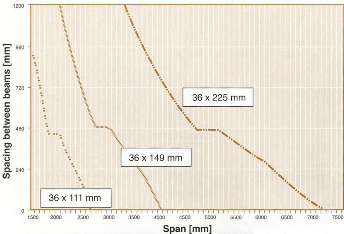
**Figure 20 Loading: Concrete tiles**
