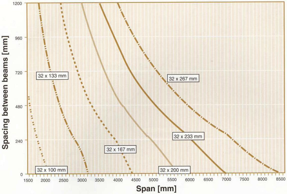
**Figure 26: Loading: Concrete tiles**
