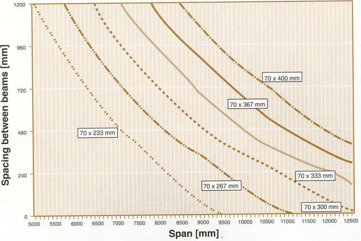
**Figure 28: Loading: Concrete tiles**
