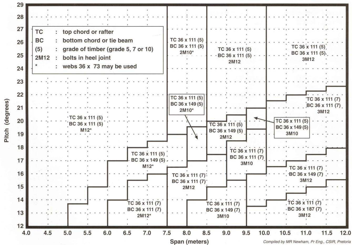
**FIGURE 2: TRADITIONAL BOLTED TRUSSES FOR SUPPORTING PROFILED METAL ROOFS: DIAGRAM SHOWING THE REQUIRED TOP AND BOTTOM CHORDS, AS WELL AS WEBS, AND ALSO ALL CONNECTING DETAILS. DETAILS ARE SUPPLIED FOR A RANGE OF SLOPES OF ROOF AS WELL AS A RANGE OF ROOF SPANS (DISTANCE BETWEEN ROOF SUPPORTS). THE TRUSSES SHOWN HERE CAN BE ERECTED AT A MAXIMUM OF 1050 MM APART.**
